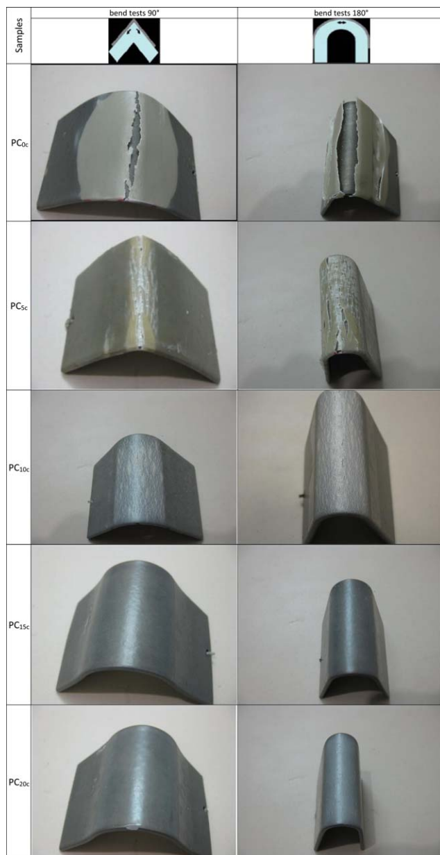
Figure 3. Macroscopic graphs of the coating samples each bended at 90° and 180° (the code of each sample is left side its photograph). [Color figure can be viewed in the online issue, which is available at wileyonlinelibrary.com .]
